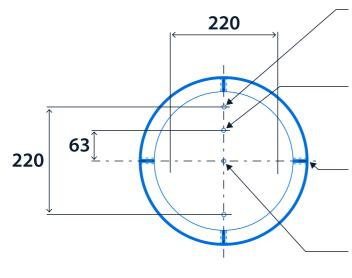
Recommended fixings - 4 x spot faces, drill as required
