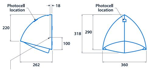
Spot marked for cable entry on both sides.
