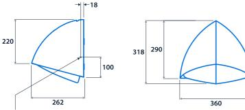
Spot marked for cable entry on both sides. Customer to drill if required.
