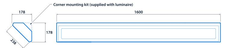
NOTE: Supply entries and fixing points to be drilled on site. IP66 integrity must be maintained
